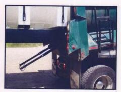
Hydraulic driven centrifugal pumps with flow rates from 82 to 210 GPM.
