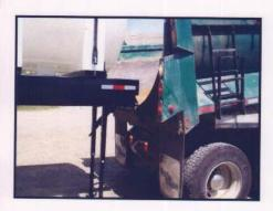
Designed for simple loading and off loading. Large roll off style rollers on front of unit reduce rolling friction. Front landing gear unlocks and folds up automatically with engagement of truck body. Unit locks into existing tailgate lock and has safety chain latches to ensure safe attachment to truck. Units made to fit U-body or Square body trucks
